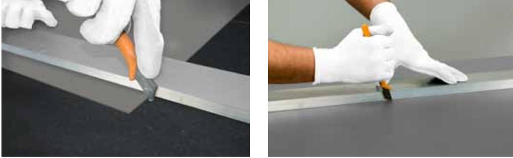
Etch the slab surface from the edge outside to edge outside, without ever detaching the blade from the etching axis and keeping it perpendicular to the surface. Do not interrupt nor restart cutting and press steadily and evenly.
