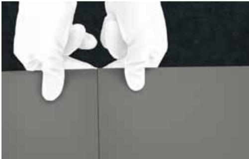
Chop off the etched surface at the edges to aid the cut fracturing. For dimensions larger than **1000 mm** open the cut by shearing from both etched edges.
