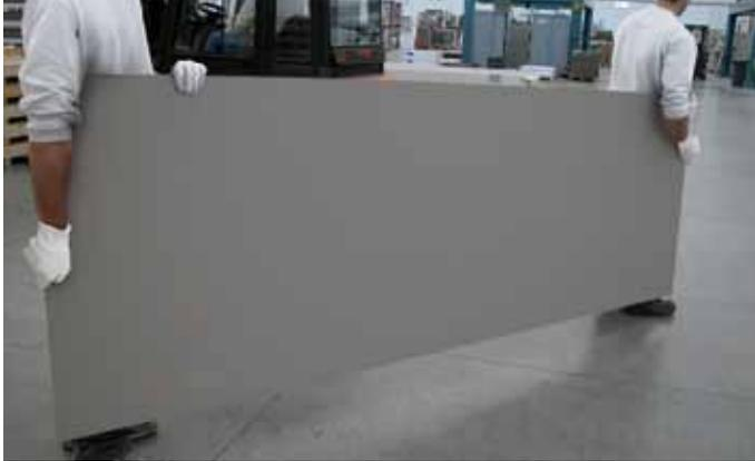
Handle the slab with the aid of a second operator, keeping it always perpendicular to the ground, without bending and protecting corners against accidental impacts.
