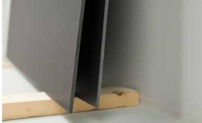
Lay the slab gently on the long side, keeping it slightly sloped and caring to arrange it on soft material or suitably spaced wooden strips.
