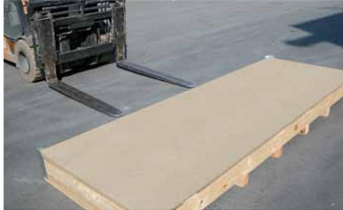
To lift and move crates of slabs **1000x3000 mm**, using fork lifts or yard cranes, it is important to get the package in the long side, caring to position in its center, extending the forks as much as possible as they have to grip all through the pallet depth.
