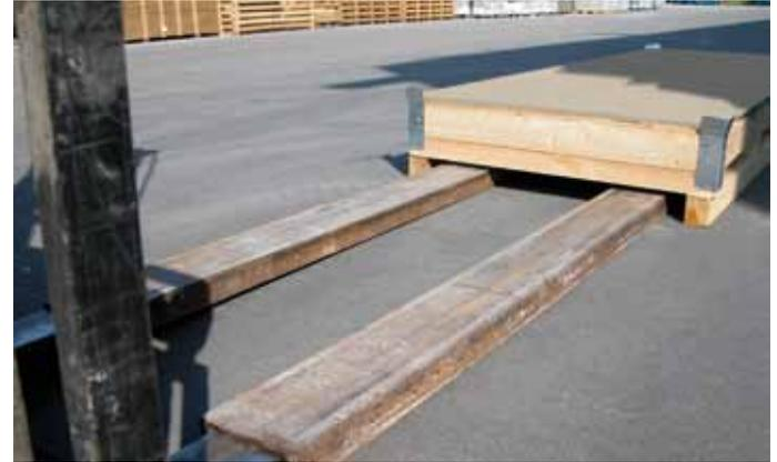
If the pallet is lifted from the short side, as it could happen while unloading from a container, min. **2.5-m** long forks shall be used for a correct product handling.
