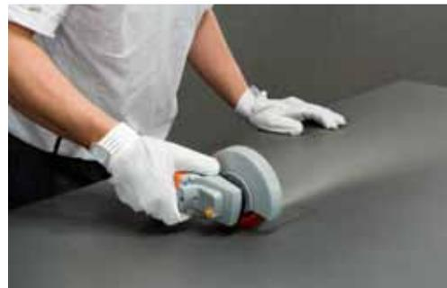
To make openings inside the slab or L-shaped cuts, use electric sanders with diamond disks with continuous band, with fast rotation speeds and low advancing speeds.
